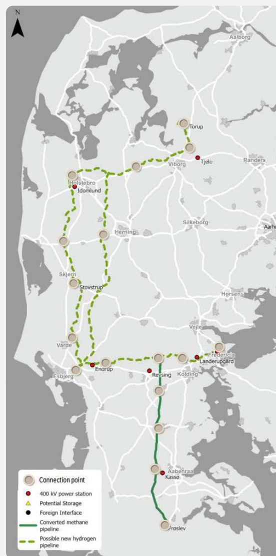
Figure 1.5: Proposed backbone routing
